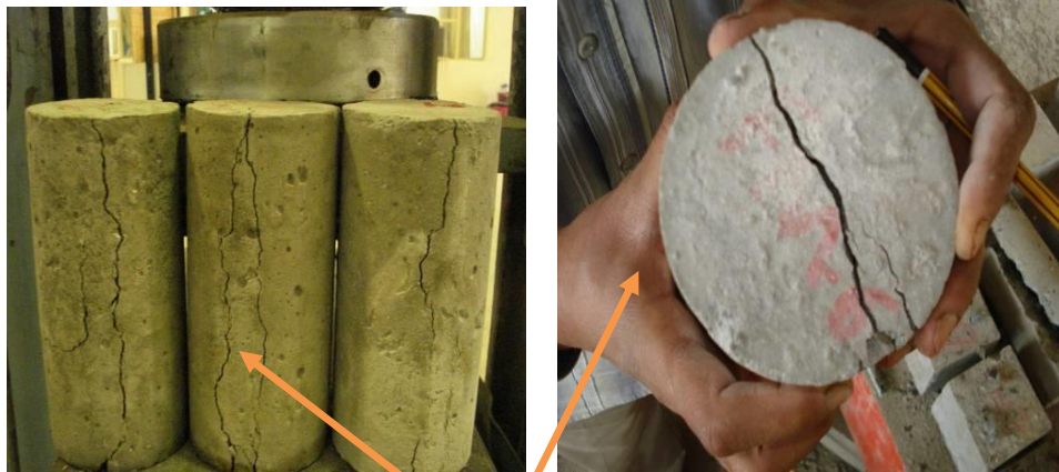
Failure in the splitting test
